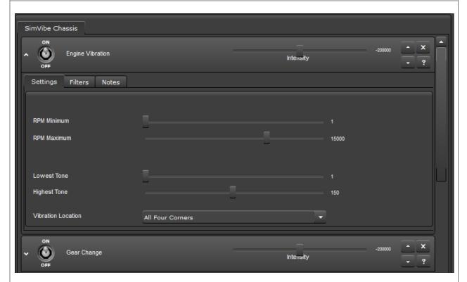
Like most SimVibe effects, you can scale the data, in this case engine rpm, into a tone (frequency). You may also choose to place the engine vibration in the front, rear or all four corners of the chassis.
