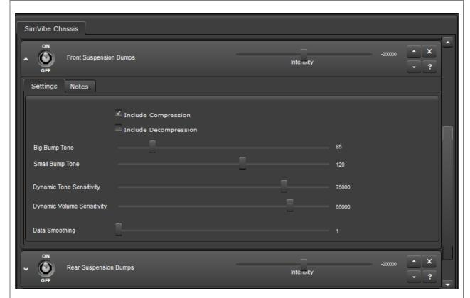
Like most SimVibe effects, you can scale the data, in this case engine rpm, into a tone (frequency). You may also choose to place the engine vibration in the front, rear or all four corners of the chassis.
