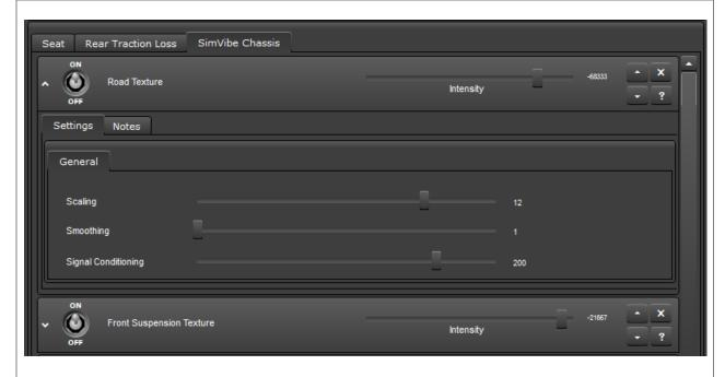
Texture based effects are not based on frequency scaling and as a result are more responsive and more able to reproduce rapid detail and texture.
